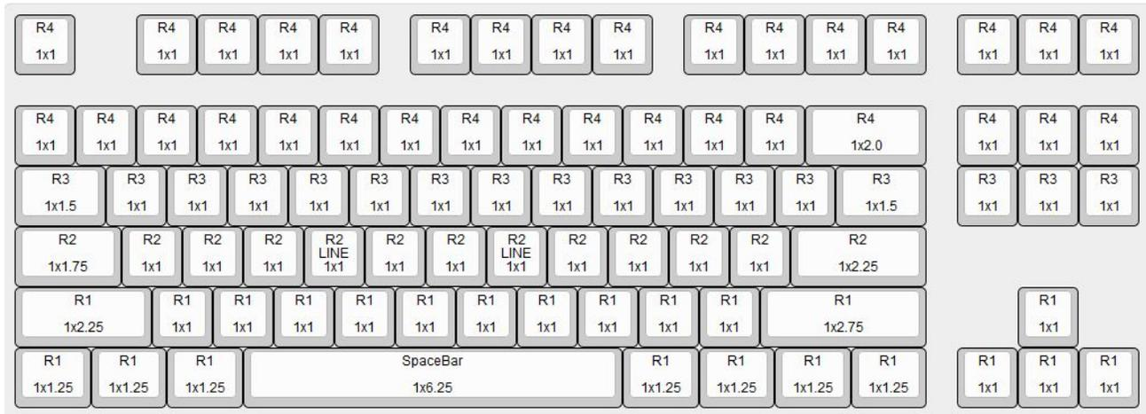
The “units” of a keycap refer to a comparison between a one “unit” standard key. This is such that a 2u key will be two units of a 1u key.
